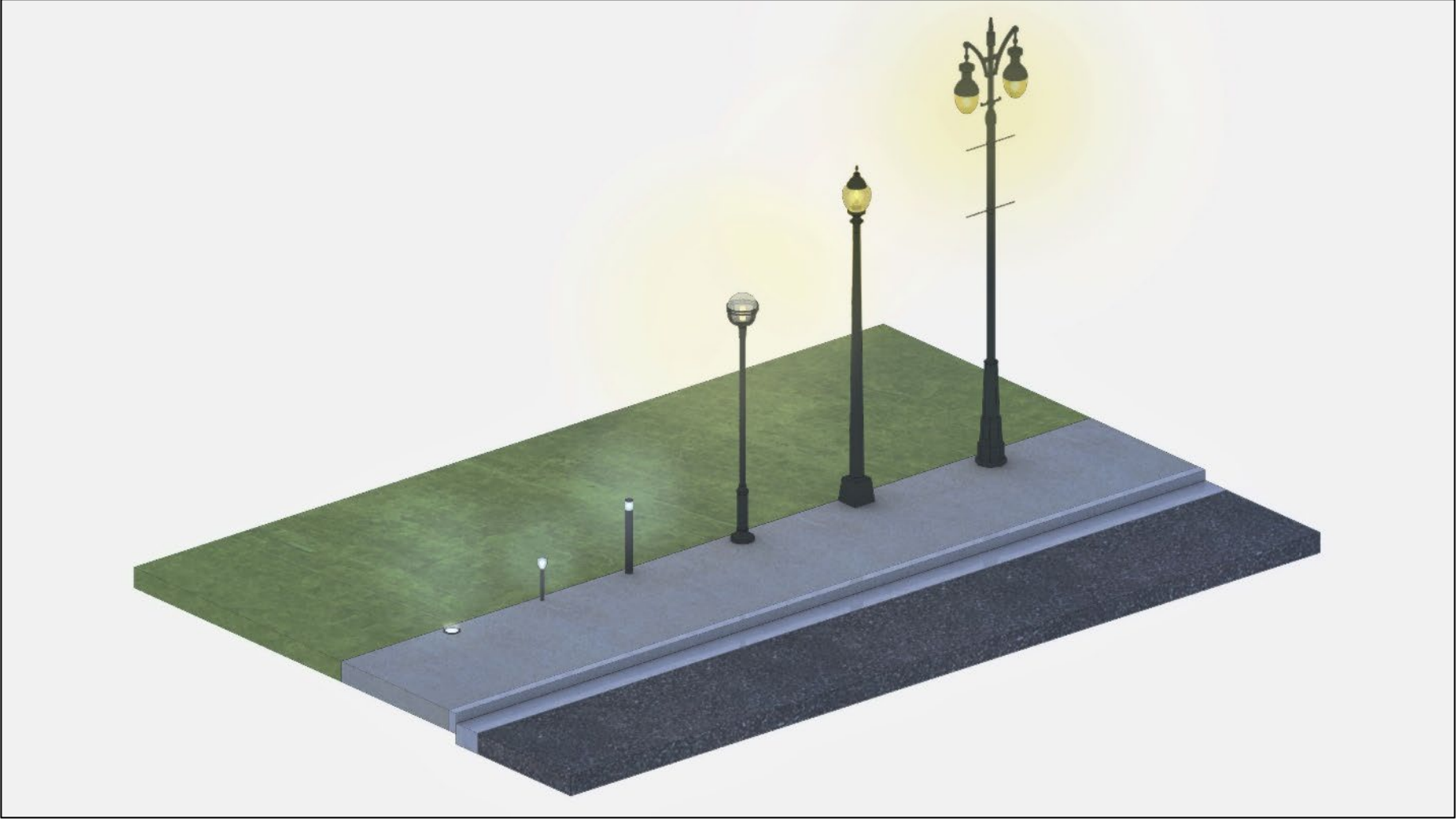
Figure 46: Non-Compliant Dark Sky Initiative Lighting Fixtures
