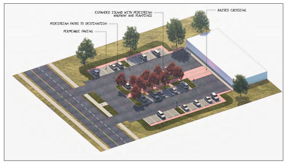
Figure 22: Example Parking Lot Enhancements – Stormwater and Pedestrian (Conceptual)
