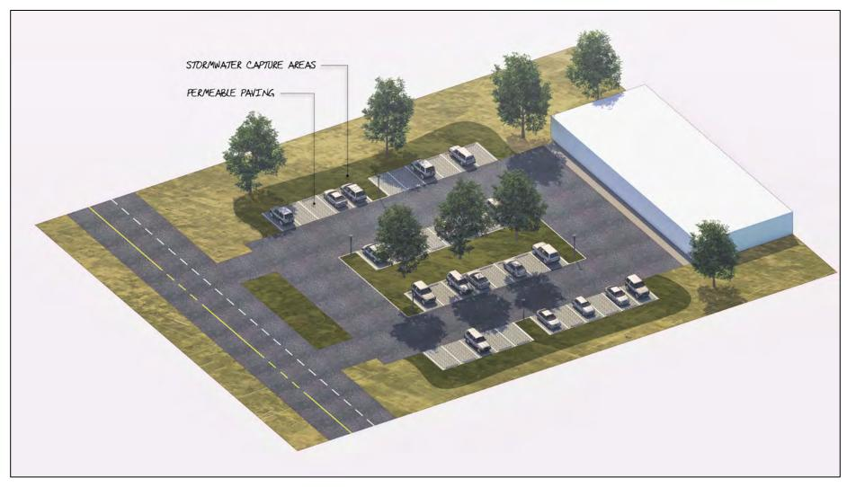
Figure 21: Example Parking Lot Enhancements – Stormwater (Conceptual)
