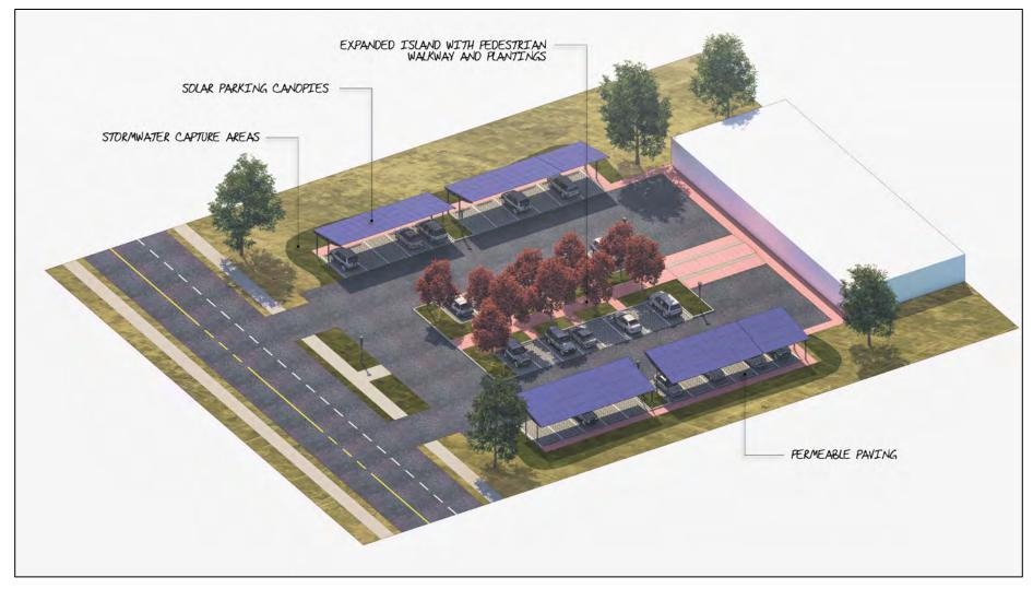
Figure 23: Example Parking Lot Enhancements – Stormwater, Pedestrian, and Heat-Reduction (Conceptual)
